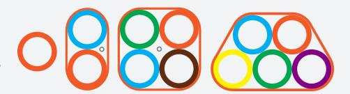
Höhle microducts are designed for long term protection of fiber optical cables. Direct Bury (DB) type of microducts are thick wall products that attain their mechanical robustness and functional performance through their intrinsic thick walls and need no further protection at underground installations. Höhle microducts conform to BS FN 61386 and BS FN 60794-5.
